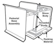
Figure 7 – Attach Pedestal to Stove Body
