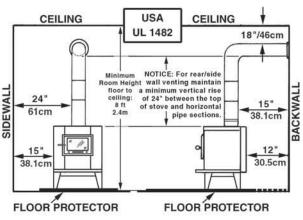
Fig. 12a – Front View Fig. 12b – Side View Minimum Clearance Dimensions from Combustible Surfaces
