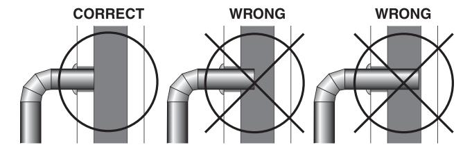
Fig. 14 - Stovepipe/Flue Connections
