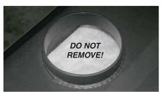
Figure 1 – DO NOT remove ceramic blanket from inside stove pipe opening. This is NOT packing material but an integral component of the stove combustion system.
