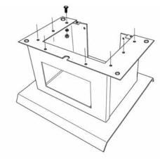
Figure 6 – Attach Pedestal Top. (Note– Position vent orifice towards front.)
