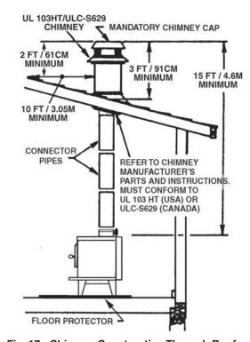
Fig. 17 - Chimney Construction Through Roof
