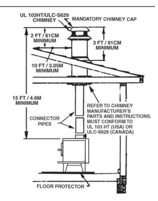
Fig. 16 - Chimney Construction Through Attic Space
