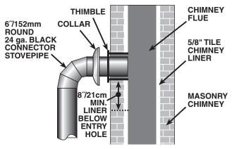
Fig.15 - Masonry Chimney Connection
