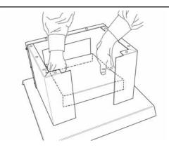
Figure 5 - Insert Ash Drawer Support.
