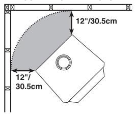
Fig. 11 – Top View Minimum Corner Clearances from Combustible Surfaces
