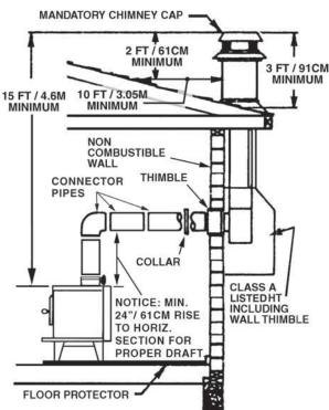
Fig. 18 - Chimney Connection to Firebox Through Masonry Wall
