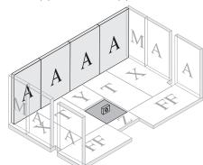
Fig. 13c- Step 3, Back Firebrick Installation Four (4) A-Size
