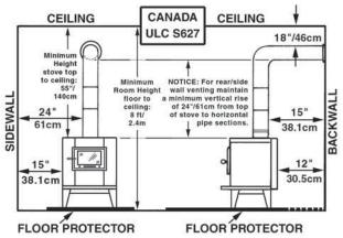
Fig. 12c – Front View Fig. 12d – Side View Minimum Clearance Dimensions from Combustible Surfaces
