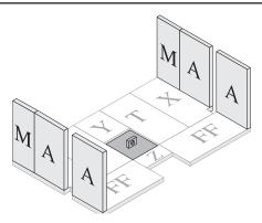
Fig. 13b- Step 2, Side Firebrick Installation Four (4) A-Size; Two (2) M-Size
