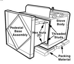
Figure 7 - Attach Pedestal to Stove Body
