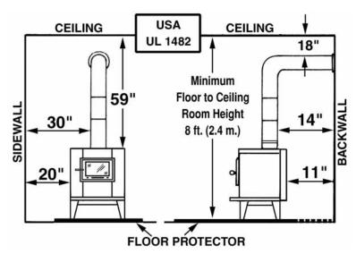
Figure 11a – Front View Figure 11b – Side View
