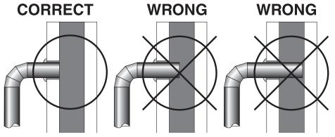
Figure 14 - Stovepipe/Flue Connections
