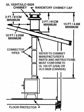
Figure 17 - Chimney Construction through Roof Chimney Minimum Height Requirements:
