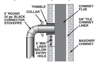
Figure 15 - Masonry Chimney Connection
