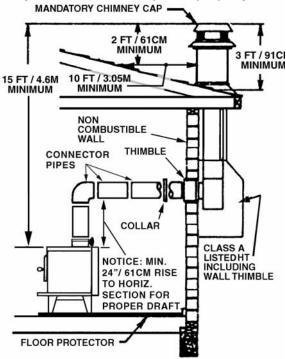
Figure 18 - Chimney Connection to Firebox through Masonry Wall
