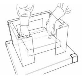
Figure 5 - Insert Ash Drawer Support.
