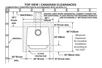
Fig. 10 - TOP VIEW Minimum Clearance Dimensions from Combustible Surfaces
