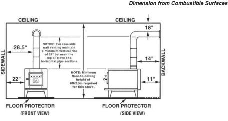
Fig. 7 – Front & Side Views: Minimum Clearance Dimensions from Combustible Surfaces
