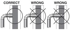
Fig.9 – Stovepipe/Flue Connections
