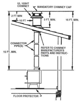
Fig. 12 - Chimney Construction Through Roof
