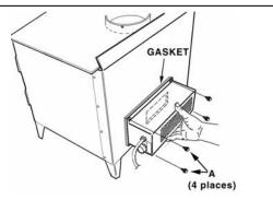
Fig. 4 – Blower attaches to rear heat deflector
