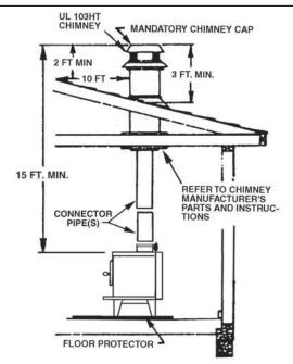
Fig. 11 - Chimney Construction Through Attic Space
