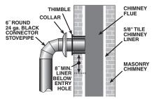
Fig. 10 - Masonry Chimney Connection
