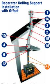
**Note:** If your Chimney runs more than 50' you must install a Roof Support # **JSC\*RS**
