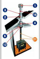
**Note:** If your Chimney runs more than 50' you must install a Roof Support # **JSC\*RS**.
