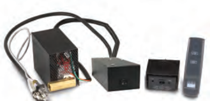
EPK-1 Automatic remote pilot lighting system. Features flame sensing pilot activation and no standing pilot. Remote control or manual option. RR-1A included.
