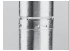
Push the ends of the pipe together.
