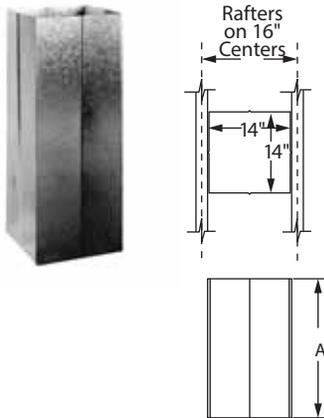
Use in installations where an 8" DuraVent chimney system passes through a roof opening with less than the normal 2" minimum clearance to roof trusses or rafters. Chimney pipe must be centered within Close Clearance Shield. (See installation instructions.)
