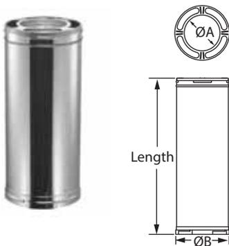
Designed for appliances tested and listed for use with wood stoves, fireplaces, furnaces, boilers, water heaters, or other appliances fueled by wood, oil, coal, or gas. 6", 9", and 12" chimney pipe has 1" insulation blanket; 24", 36" chimney pipe has 1/2" insulation. To calculate the installed length of DuraPlus chimney pipe, subtract 1 1/2" from each length of chimney pipe.
