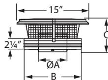
Required where chimney pipe terminates above the roof line. Removable screws allow for cleaning of the chimney and spark arrestor screen. Made of stainless steel.
