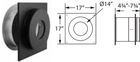
Adjusts from a minimum of 4 3/4" to a maximum of 7 3/4" wall thickness, and fits between standard wall studs. To accommodate thicker walls, the telescoping pieces can be extended up to 16" with a field-fabricated extension installed. Interior trim ring painted black. Must be installed with DuraPlus chimney pipe horizontally through the wall and extend a minimum of 2" into the room beyond the interior wall. For adapters, see DVL and DuraBlack section.
