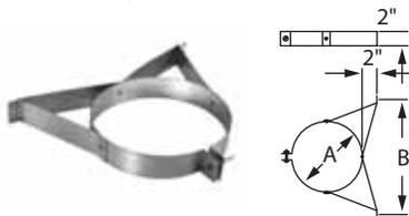
Use in interior or exterior installations to support and to stabilize the chimney while assuring a 2" clearance. Wall straps are required every 4' on exterior of building only.
